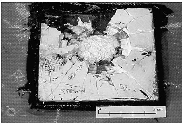
Fig. 3. Formation of fractured cone showing lateral spread of ceramic fragments.
