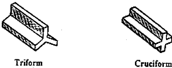
Figure 5. Novel Penetrator Geometries From Bless et al. (1995).
