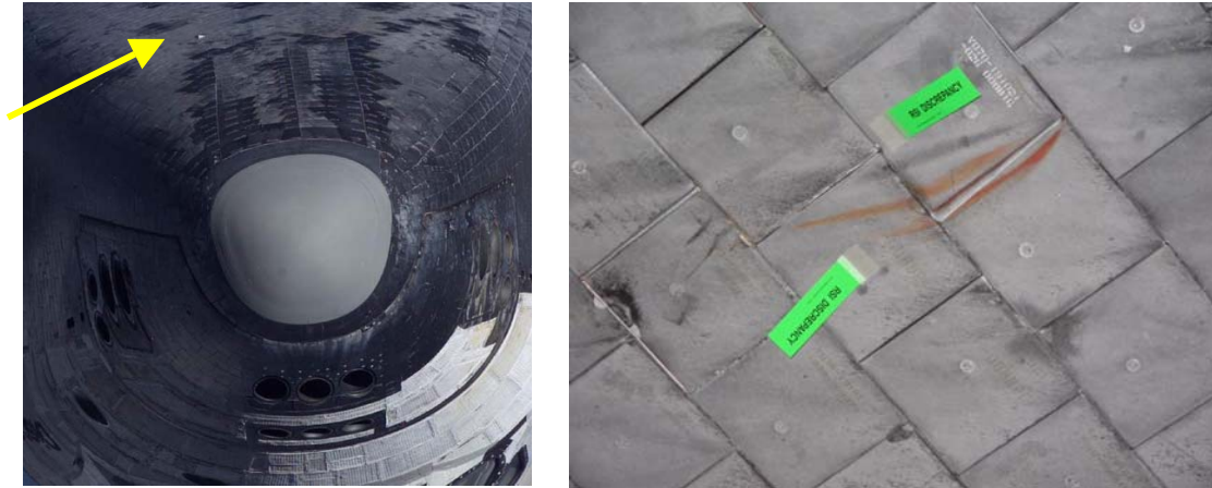
Figure 1. Left: protruding gap filler (protruding about 2.8 cm or 1.1") observed on the underside of the space shuttle Discovery as seen from the International Space Station, later removed by an astronaut during a spacewalk (STS-114, photo ISS011e11074); right: re-entry scorch marks on Discovery underside near a protruding gap filler on the next flight (STS-121 after landing, author photograph during post-flight inspection).
