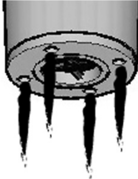
Figure 2. Properly located/pointed high-velocity jets might be used to control the main flow around the base region and in this way somewhat higher drag reduction might be obtained.
