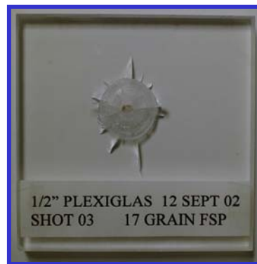
Figure 5: Experimental impact at 846 m/s
