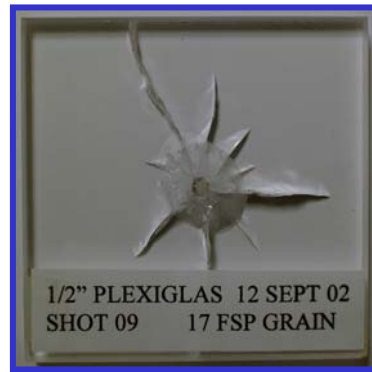
Figure 3: Experimental impact at 475 m/s
