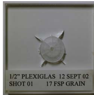
Figure 7: Experimental impact at 1004 m/s
