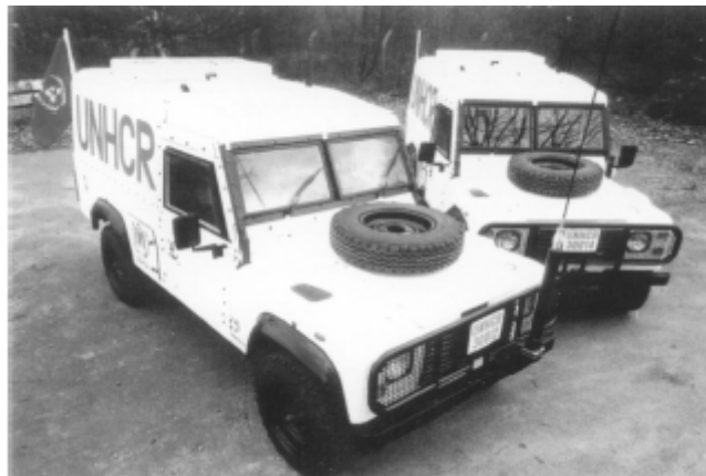
Figure 3 Armoured Land Rovers (CAV-100) with body armour based on S-2 glass fibre panels produced by National Plastics.
